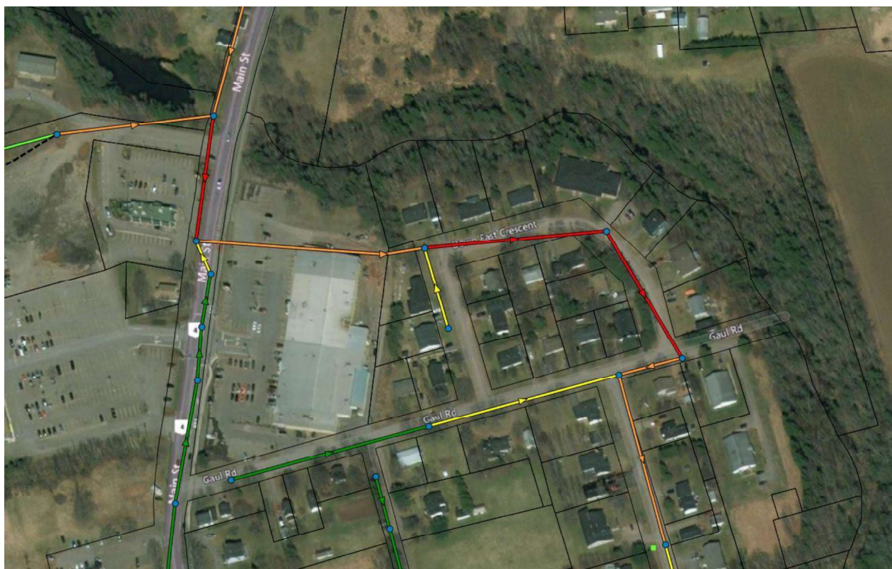
Figure 3.4: Main Street 200mm Sewer and Down East Crescent 250mm Sewer Showing Over 80% Full Under Infill Plus Extension to MacDonald Road Growth Scenario
