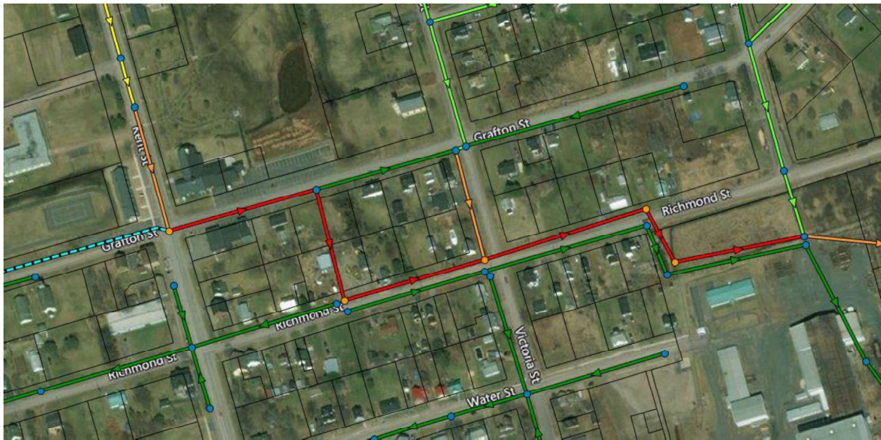
Figure 3.7: Existing Section of 250mm Sanitary Main Surcharging Under the Full Buildout Development Scenario
