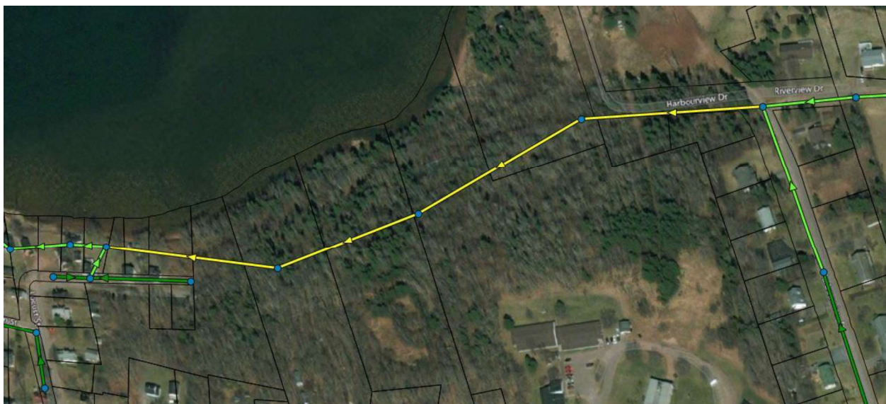
Figure 3.1: Existing 200mm Sanitary Trunk Sewer along the River to the Montague WWTP
