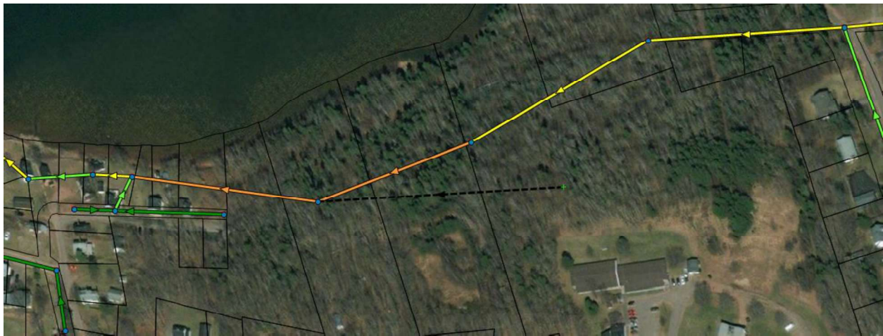
Figure 3.3: Existing 200mm Sanitary Trunk Sewer along the River to the Montague WWTP Under Infill Growth Scenario Flows
